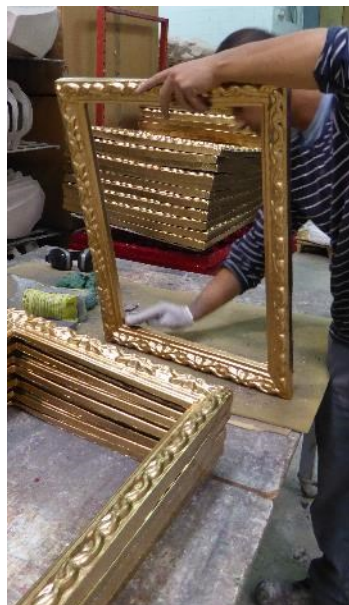
The frames were painted with 3 coats of paint to ensure brightness and durability.
