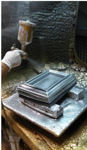
The frames were painted with 3 coats of paint to ensure brightness and durability.
